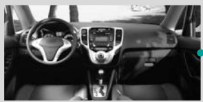
Instrument Panel - Soft Type : PP+LGF20
