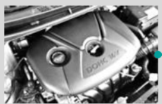
Engine Cover - PP+LGF+Glass Bubble
